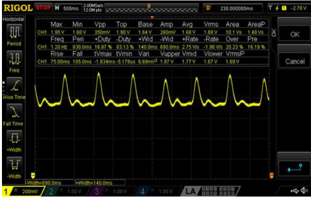
Fig. 4. Oscilloscope reading of the heart rate pulse
